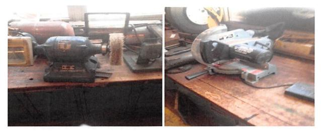
OSHA 29 CFR 1910.212- Machine Guarding- Machines designed for a fixed location shall be securely anchored to prevent walking or moving. If miter saw and grinder are permanently station in this area ensure they are properly anchored.
