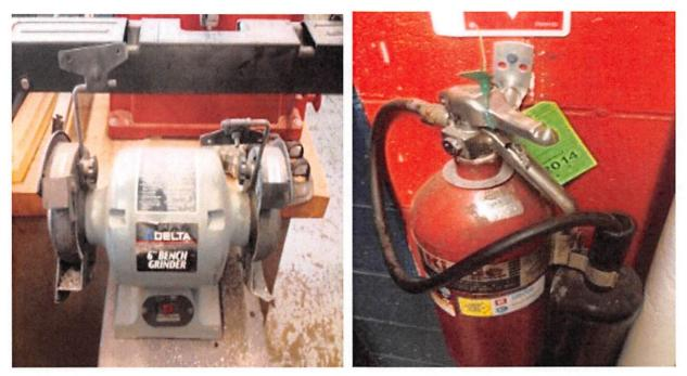
The pictured bench grinder is missing tool rests and a shield. If this piece of equipment is currently in use, the safety modifications need to be made prior to student use.
